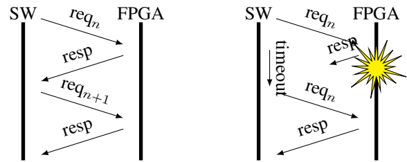
Fig. 4. Sequence diagram of the communication protocol.
